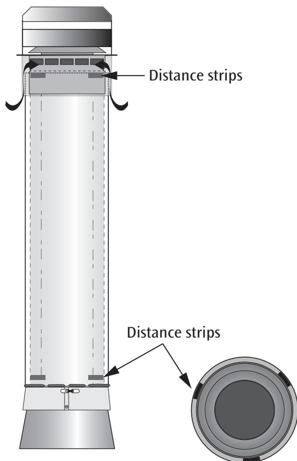
An extra cladding pipe with a dimension of  $\text{Ø}275$  is supplied with the delivery of NVI2000 Combi when a round chimney hood is selected. The function of the pipe is to minimise the risk of condensation.
