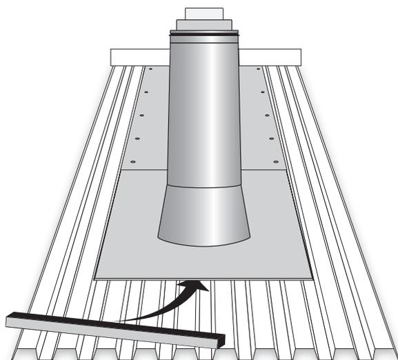
For roofs made of metal, the roof seal must reach up to the roof ridge. If this is not satisfied, extension plates must be used.
