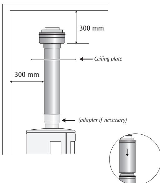
Start by measuring the hole in the ceiling based on the fireplace's flue connecting piece. Cut out the hole in the ceiling to ensure the correct safety distance to any flammable material.
