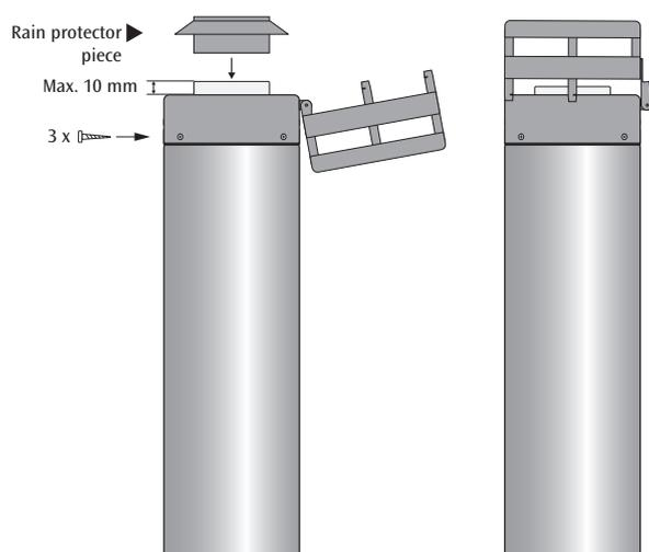
Place the rain/top protection on the uppermost module pipe, secure with the three enclosed screws, as illustrated. The protection must be installed so that it is level with the inner pipe.\*
