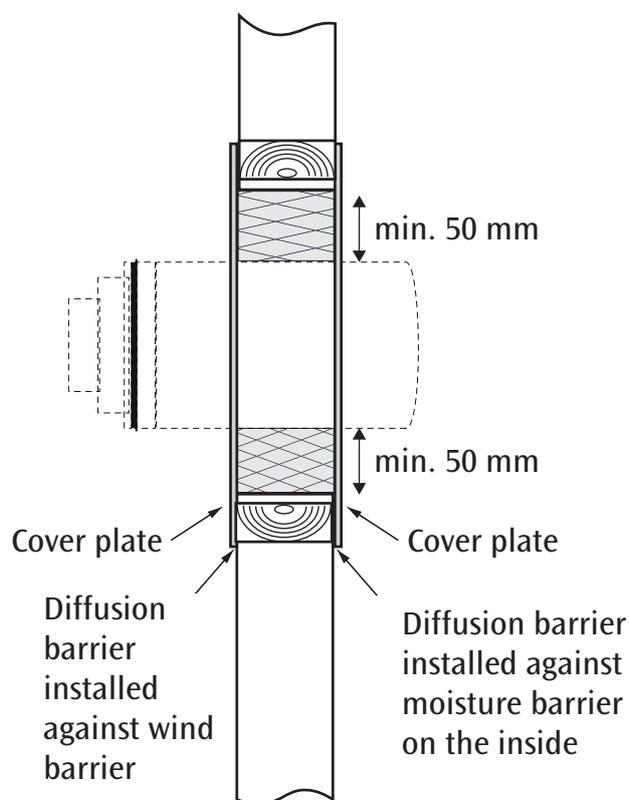
In the case of a through-connection in a wall where the insulation material comprises chipboard, loose wool or equivalent, a shaft must be built with measurements in accordance with the table on page 5.
