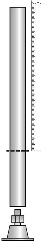
Start by measuring the distance from the floor to the middle of the fireplace's rear connecting piece.
