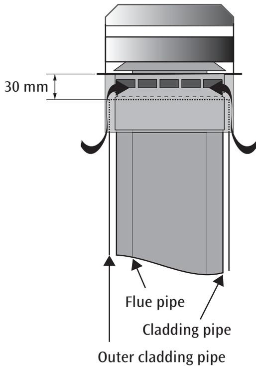
When adapting the chimney length, it is important to ensure that the supply air is able to pass freely through the top of the chimney. Leave a distance of at least 30 mm between the roof and the end of the cladding pipe.
