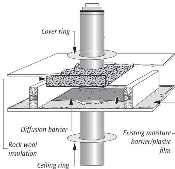
Fully insulated chimney passes through a flammable floor structure, up to 300 mm insulation with required distance without accessories. Rock wool insulation (supplied with ceiling ring) is then used next to the ceiling.
