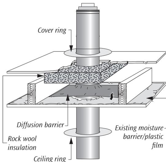
If fully insulated Combi modules are used, no additional insulation is required. However, bear in mind that the safety distance of 50 mm to flammable materials must always be observed.
