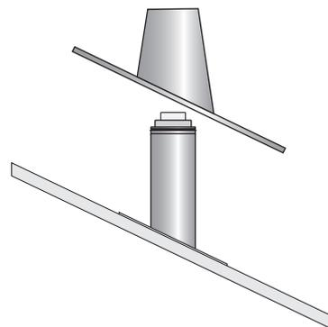
*Thread the roof seal over the chimney module, and lower it carefully towards the roofing tiles (so that the system chimney's paintwork does not sustain any damage).*
