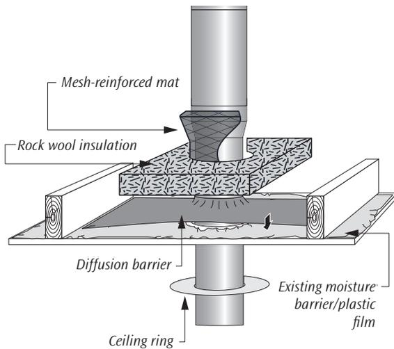
If a semi-insulated module ends up fully or partially in the joisting, it must be provided with additional insulation with a 30 mm thick, mesh-reinforced mat that comes with the adapter.
