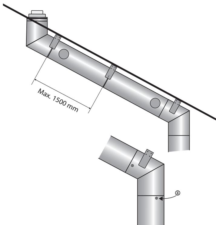
If the pipe is angled more than 45° from the vertical, or if the distance between 15-45° bends is more than 200 cm, a cleaning hatch is required. The max. distance between cleaning hatches is 5 meter.
