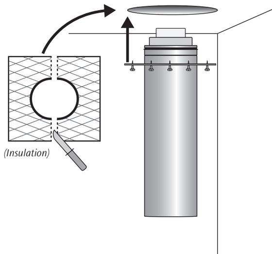
Cut a hole in the insulation panel that is supplied with the ceiling plate. The hole must be the same size as the cladding pipe. Cut the panel in half and insert the pieces up into the floor structure around the chimney.
