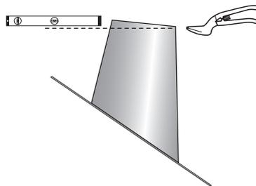
If the cone's opening does not correspond with the roof angle, cut it horizontally before screwing the cone/roof seal into place.
