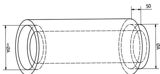
When there is a requirement to adapt the length of modules, all components must be cut by the same amount.
