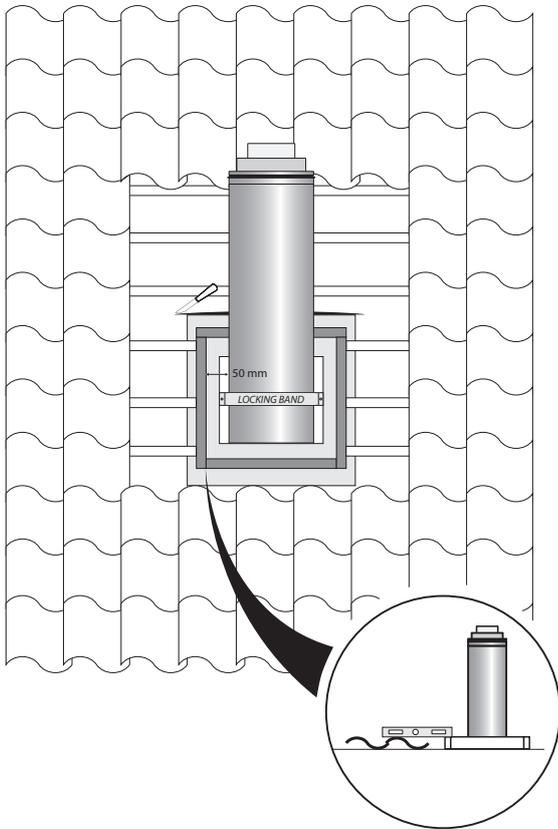
Check the surface after making a hole in the roof and make sure that the bottom fitting has a load-bearing, stable attachment. If not, build a frame attachment.
