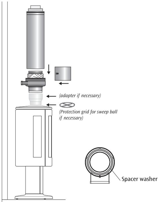
Start the installation with the connecting piece, install the rectangular connecting piece in the direction in which the connection duct is subsequently to be installed.
