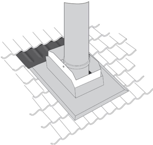
Build a frame around the bottom fitting's connecting piece at the same height as the roofing. Return the cornice and then the roofing. In some cases, it may be necessary to cut roofing tiles.
