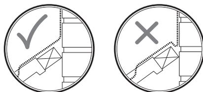
There must not be any pockets where standing water can collect. This is particularly important at the top edge. It may be necessary to install bushings here of the same height as the top of the profile on the roofing.
