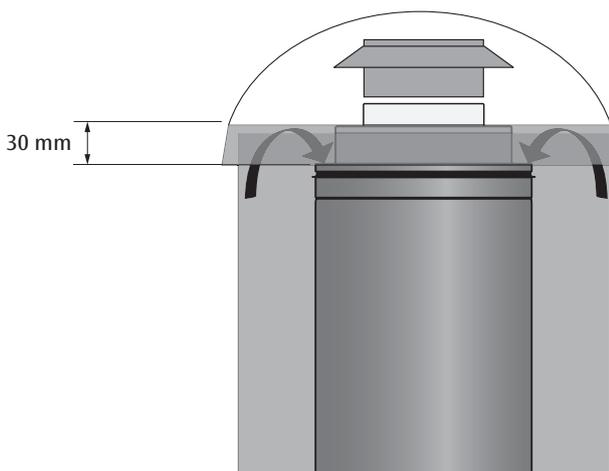
When adapting the chimney length, it is important to ensure that the supply air is able to pass freely through the top of the chimney. Leave a distance of at least 30 mm between the roof and the end of the cladding pipe.
