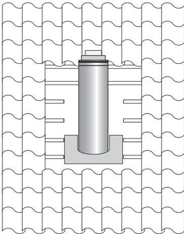
After making a hole in the roof, inspect the surface and make sure that the stay plate is supplied with a load-bearing, stable attachment. If not, build a frame for attachment.
