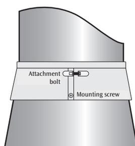
Place the vulcanising tape over the roof seal and module pipe in order to seal the gap that arises. The tape must be stretched so that there is pressure around the entire chimney.
