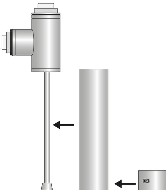
The length of the cladding pipe must be adapted to the existing installation.
