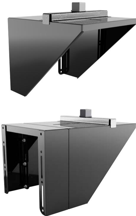
The wall bracket comes with a pre-installed load-bearing plate. This distributes the load out towards the stronger edges. The load-bearing plate must be used when installing through an outer wall.
