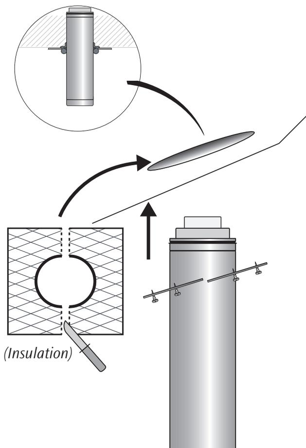
Cut a hole in the insulation panel that is supplied with the ceiling plate. The hole must be the same size as the cladding pipe. Cut the panel in half and insert the pieces up into the floor structure around the chimney.
