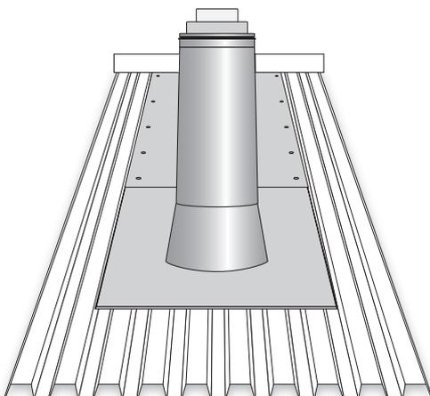
In the case of a steel plate roof, the lower fitting must extend in under the next steel plate joint with a minimum overlap of 10 cm or up to the roof ridge. If this is not satisfied, extension plates (accessories) must be used.
