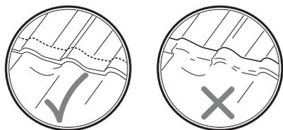
The membrane must not end with an open edge facing the roofing at the top edge. It must be inserted underneath to ensure an overlap, at least 10 cm.
