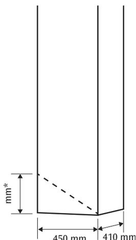
The casing comprises four plates and one stay plate. The plates for the casing are attached with the aid of a “snap lock” and cannot be separated once they have been assembled, so make sure that the ends of the plates are completely even before you assemble them.
