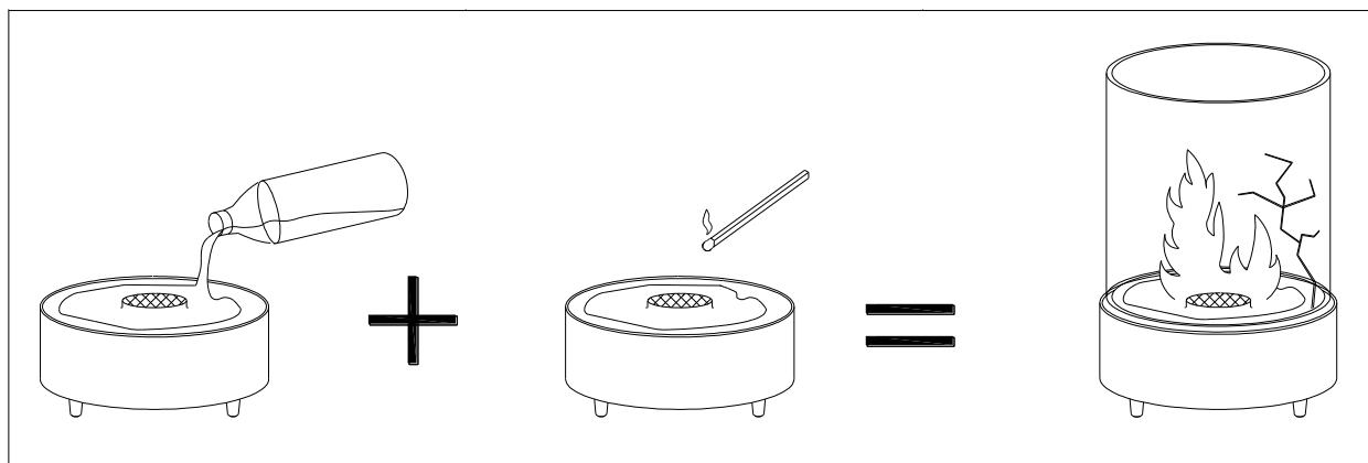
**EN** Igniting the spilled fuel is extremely dangerous and will cause the glass tube to crack. **Glass tube is not covered by the warranty.**
